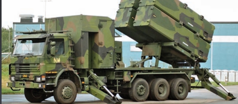
Scania P113HK8x6HZ (8x6) 3 Series carrier/launch truck for four land-based Saab RBS-15 anti-ship missiles.
