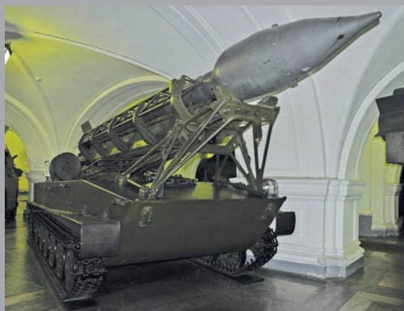
Top right: the 2P27 was the first ATGM vehicle mounted on the BRDM chassis.
