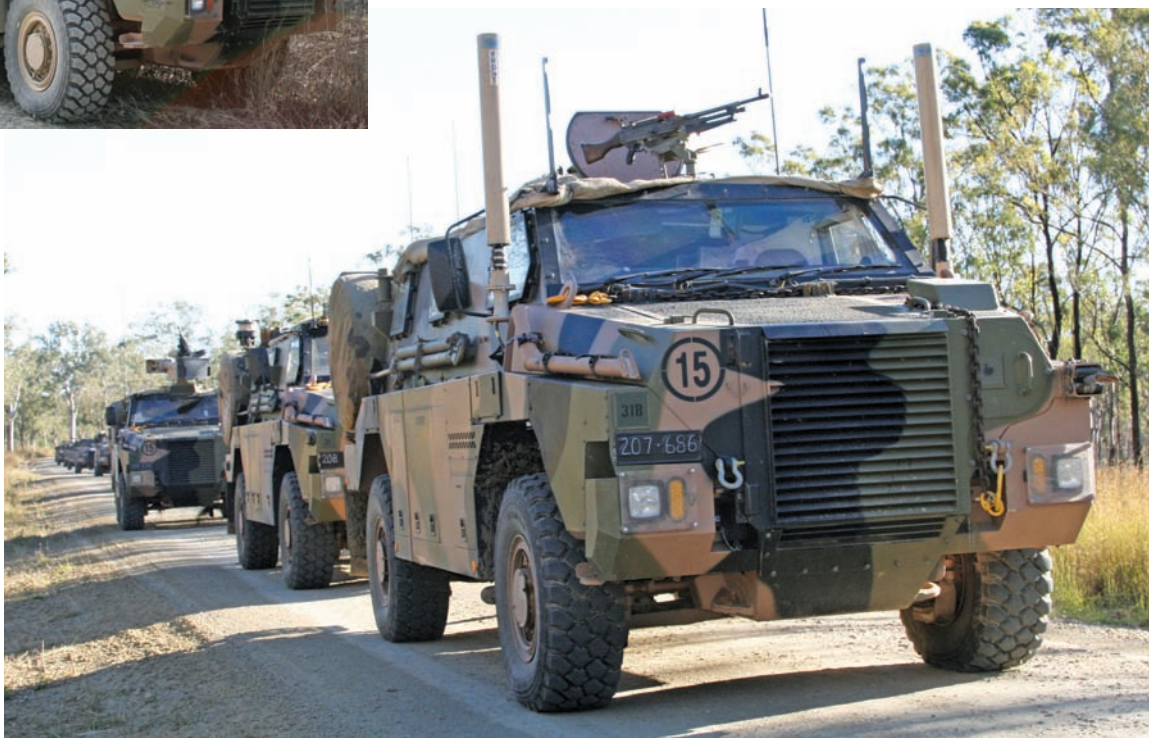
Top left: the 7.62mm MAG 58 serves as the standard GPMG in the Australian Army, and here one is fitted in the R-400 RWS. Alternatively a .50-cal MG can be fitted.
