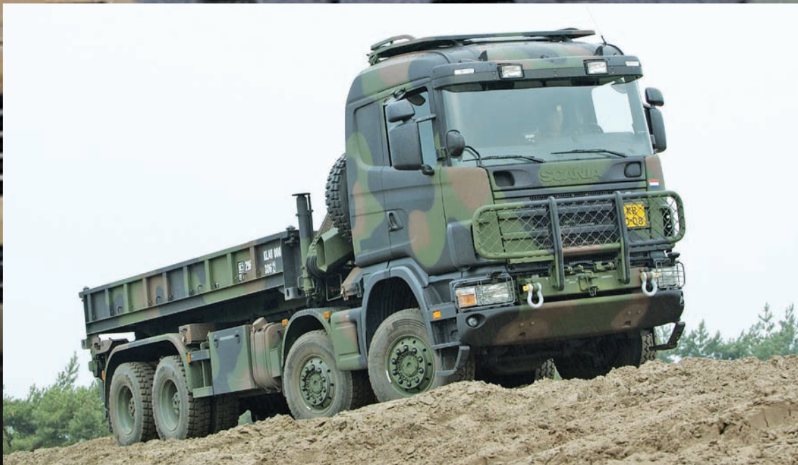
Left: the P124CB8x8HZ420 (8x8) 4-series truck is based around Scania's commercial trucks and the modular use of components from these. The Dutch Army have received 555 examples (2005/2006), the Swedish 66 (2001) and the Irish 15 (2004/2005); there are slight specification variances between the three deliveries.
