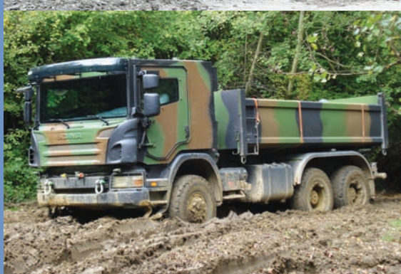
Scania P113HK8x6HZ (8x6) 3 Series carrier/launch truck for four land-based Saab RBS-15 anti-ship missiles.
