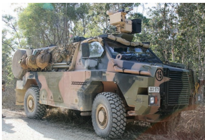
Top left: the 7.62mm MAG 58 serves as the standard GPMG in the Australian Army, and here one is fitted in the R-400 RWS. Alternatively a .50-cal MG can be fitted.
